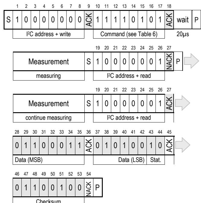
**Figure 16** No Hold master communication sequence – grey blocks are controlled by SHT2x. If measurement is not completed upon "read" command, sensor does not provide ACK on bit 27 (more of these iterations are possible). If bit 45 is changed to NACK followed by Stop condition (P) checksum transmission is omitted.
