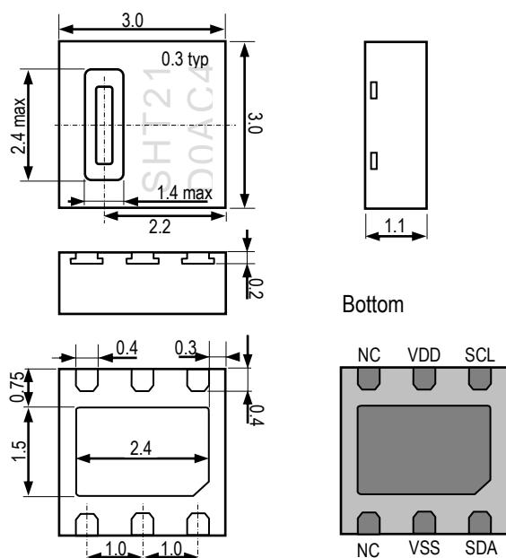
**Figure 1:** Drawing of SHT25 sensor package, dimensions are given in mm (1mm = 0.039inch), tolerances are  $\pm 0.1$ mm. The die pad (center pad) is internally connected to VSS. The NC pads must be left floating. VSS = GND, SDA = DATA. Numbering of E/O pads starts at lower right corner (indicated by notch in die pad) and goes clockwise (compare Table 2).
