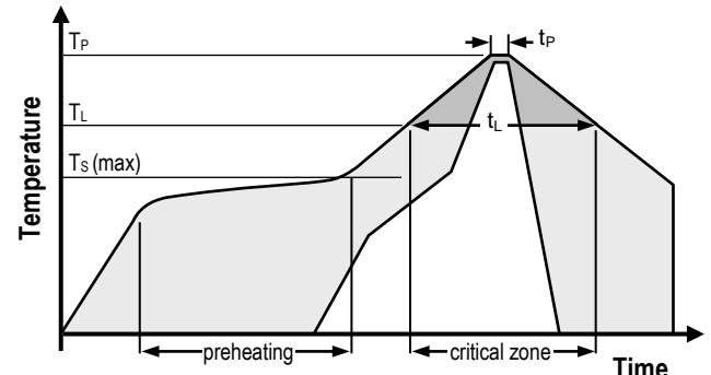
**Figure 9** Soldering profile according to JEDEC standard.  $T_P \leq 260^\circ\text{C}$  and  $t_P < 30\text{sec}$  for Pb-free assembly.  $T_L < 220^\circ\text{C}$  and  $t_L < 150\text{sec}$ . Ramp-up/down speeds shall be  $< 5^\circ\text{C/sec}$ .
