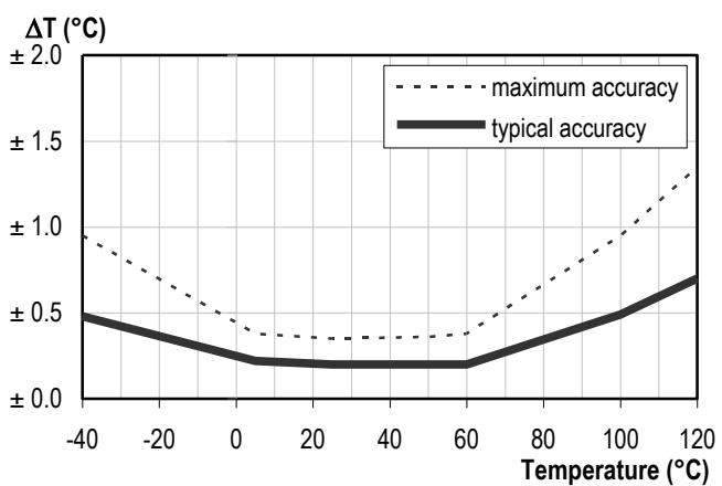
Figure 3 Maximal tolerance for temperature sensor in °C.
